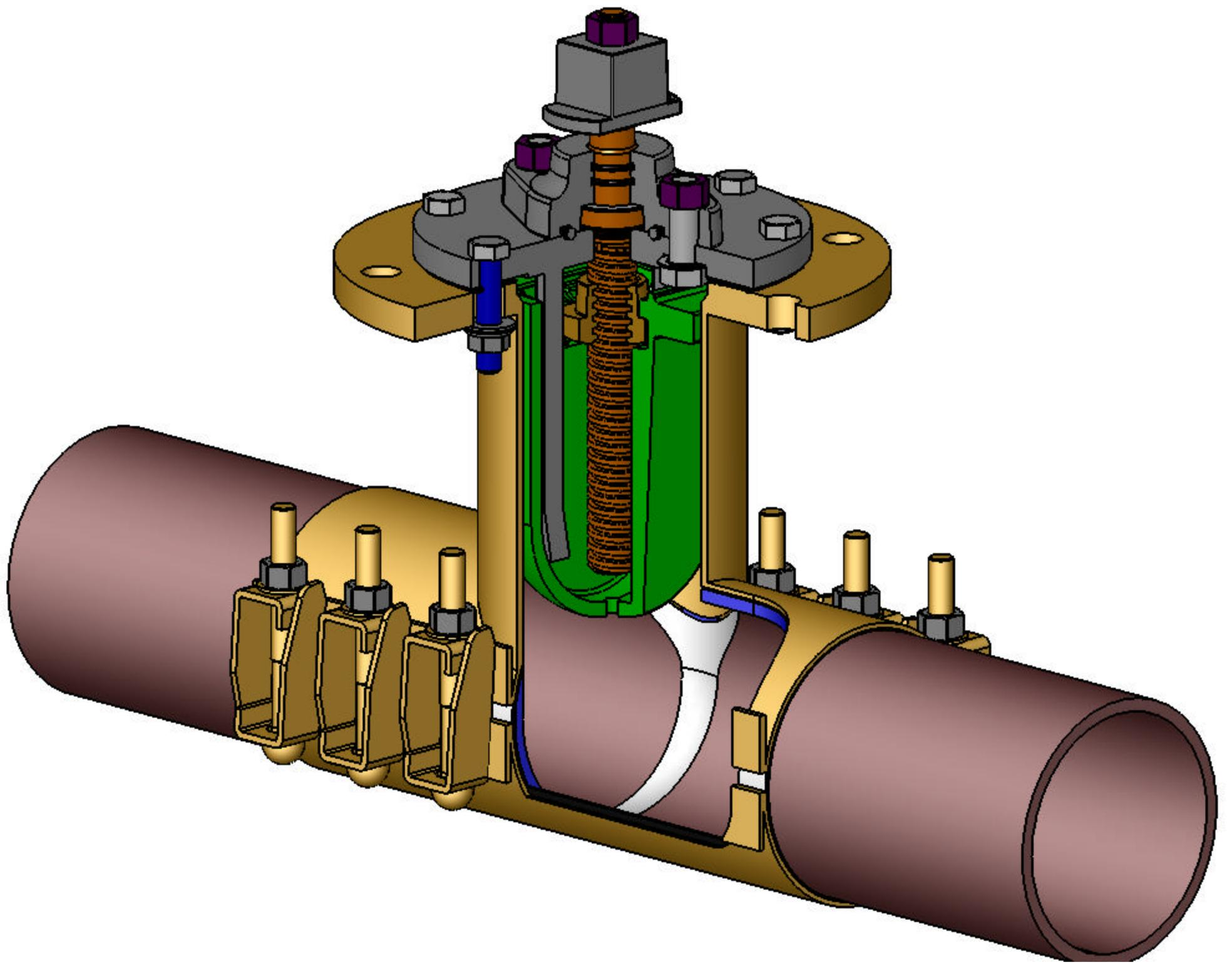
The QuikValve Sleeve shall be fabricated to assure a 360° seal around the pipe under working pressures up to 150 psi (test pressure: 225 psi). The sleeve will be made of ASTM A-36 steel, lined and coated with fusion bonded epoxy to 10-12 mils. Epoxy to meet the requirements of AWWA C-213. Provides attachment to pipe for drilling, reaming and final assembly of the QuikValve Water Control Valve. May be used on cast iron, ductile iron, asbestos cement, C900 PVC and some IPS PVC pipes.
